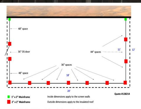
Walls are 8' tall with an 18" kickplate. Single outswing door quoted. Insulated roof is 4" thick
